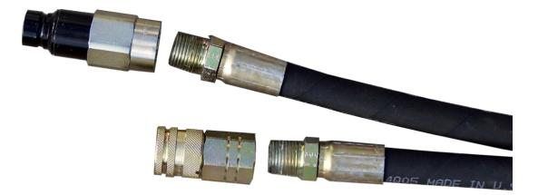
• Once the couplers are installed, you may connect them to your machine by pushing the male coupler into the female coupler on the Skid Steer and the female coupler of the attachment into the male coupler on the Skid Steer.
